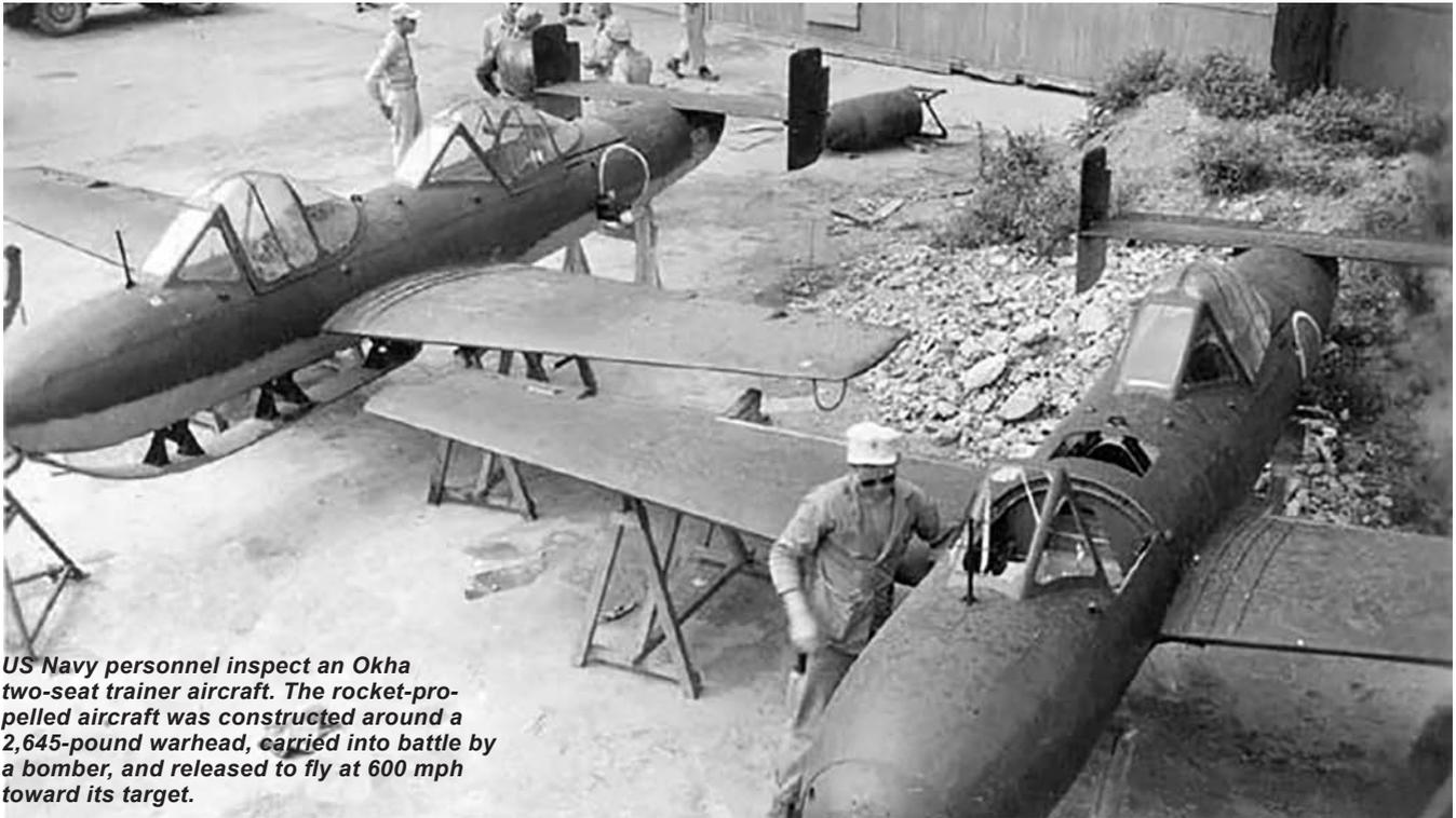
**US Navy personnel inspect an Okha two-seat trainer aircraft. The rocket-propelled aircraft was constructed around a 2,645-pound warhead, carried into battle by a bomber, and released to fly at 600 mph toward its target.**
