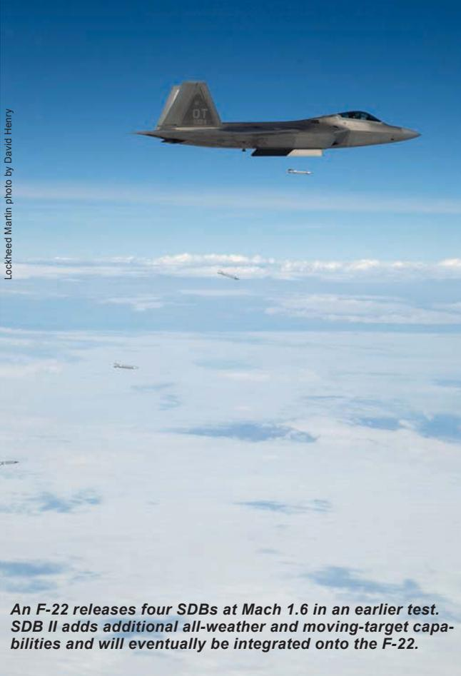
**An F-22 releases four SDBs at Mach 1.6 in an earlier test. SDB II adds additional all-weather and moving-target capabilities and will eventually be integrated onto the F-22.**
