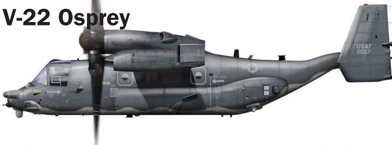
The V-22 Osprey “tilt-rotor” is a unique multimission aircraft capable of vertical and short takeoff and landing. Typically, it takes off and lands like a helicopter. However, when airborne, its engine nacelles and 38-foot, three-bladed proprotors can rotate forward 90 degrees for horizontal flight, converting the Bell Boeing aircraft into a more fuel-efficient, higher-speed turboprop aircraft.
