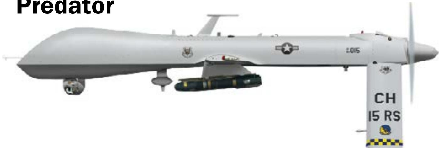
Predator, a remotely piloted aircraft, became world famous as the first successful weaponized RPA and first to conduct lethal strikes. Designed by General Atomics Aeronautical Systems, this medium-altitude, long-endurance system was first used by USAF for surveillance. Later it was armed with laser guided missiles and flown against terrorist targets. Many lethal missions were CIA ventures, but the aircraft, pilots, and command and control systems belonged to the Air Force.
