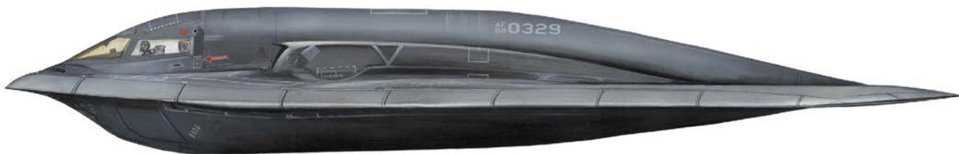
The B-2 Spirit entered USAF service in 1993 as the world's first "stealth" bomber. This long-range, four-engine, subsonic Northrop aircraft was a flying wing, with no fuselage or tail. It drew its stealthiness from extremely low radar, acoustic, infrared, and visual signatures, plus advanced avionics. These, in combination, thwarted detection and tracking systems that might have allowed a foe to direct missiles or interceptors against it.
