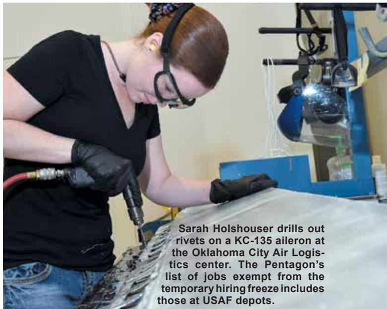
Sarah Holshouser drills out rivets on a KC-135 aileron at the Oklahoma City Air Logistics center. The Pentagon's list of jobs exempt from the temporary hiring freeze includes those at USAF depots.
