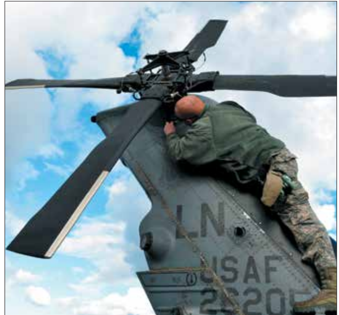
A maintenance crew chief with the 56th Rescue Squadron, US Air Forces in Europe, works on an HH-60G Pave Hawk anti-icing component.
