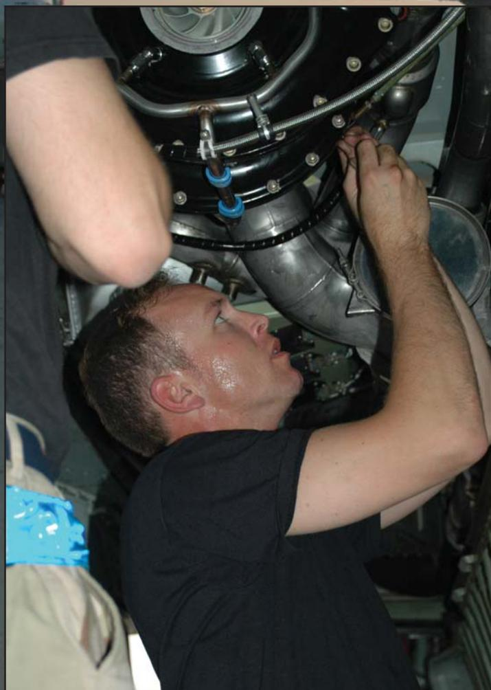
Staff Sgt. Kevin Tarwater, electronic warfare systems craftsman with the 55th Aircraft Maintenance Unit, replaces an air cycle machine which is used as one of the primary means to cool the aircraft cabin.
