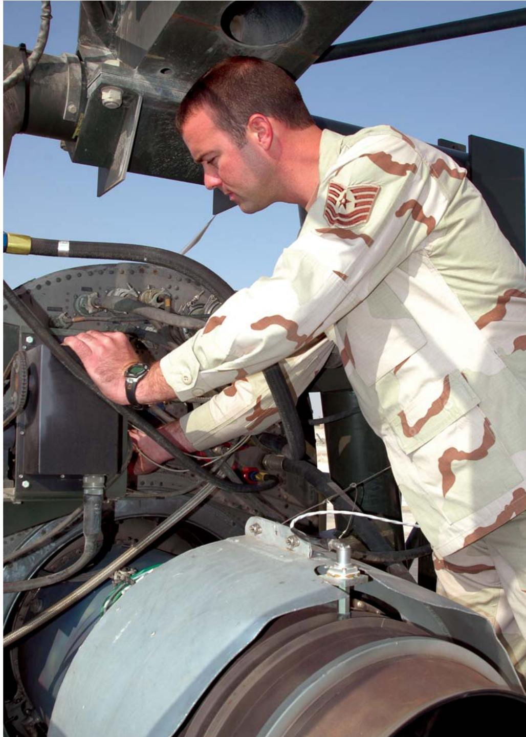
**Tech. Sgt. Robert Moore, Centralized Intermediate Repair Facility test cell section chief, looks at a T-56 engine used on C-130s before running tests on it at the newly built engine test cell facility.**
