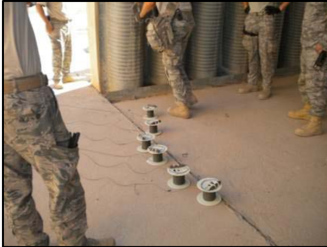
Figure 2: Placement of shock tube and initiators
