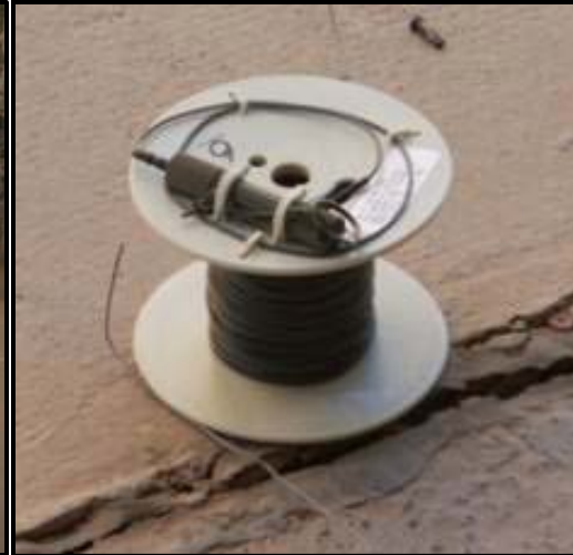
Figure 3: Close up view of shock tube and detonation initiator
