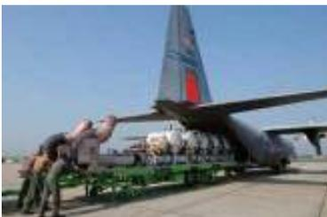
*Airmen from the North Carolina Air National Guard's 145<sup>th</sup> Airlift Wing push a modular airborne fire fighting system onto a C-130 Hercules. The system is a series of pressurized tanks that hold 3,000 gallons of flame-retardant liquid. The retardant is dropped along the leading edge of a fire to block the spread of flames.*
