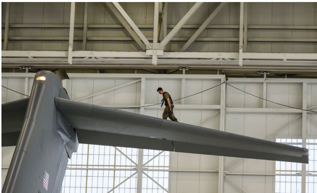
Staff Sgt. Mitchell Halbleib, 60th Maintenance Squadron, ensures the proper operation of elevator systems on the tail of a C-17 Globemaster III at Travis Air Force Base, Calif.
